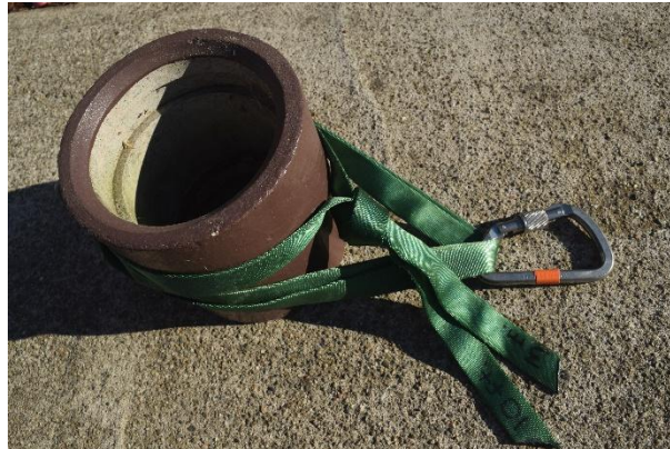
W3-P2 with flat overhand bend
