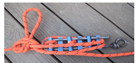
modified rack tie-off
