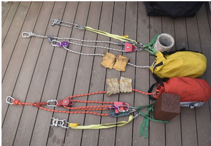
DCTTRS raising with a 3:1 and a 5:1 system
