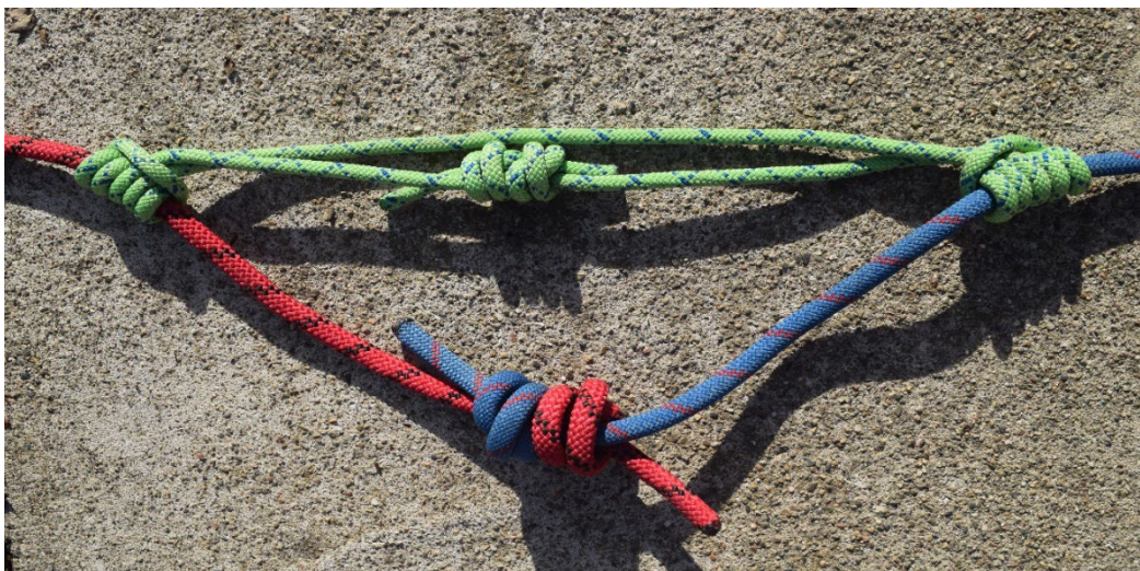
soft interface joining ropes
