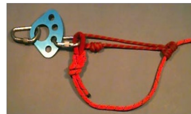
soft interface at end of rope
