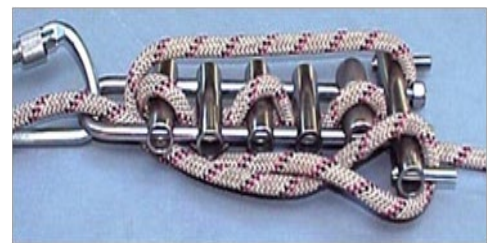
U-shaped rack tied off
