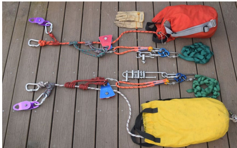
two tensioned rope system
