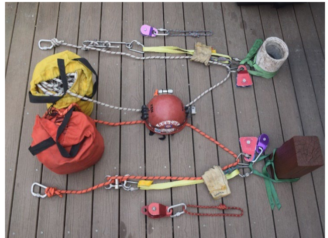
DTTRS lowering with a rack and a Scarab™
