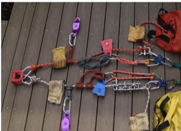
two tensioned rope system lowering with Scrabe and rack
