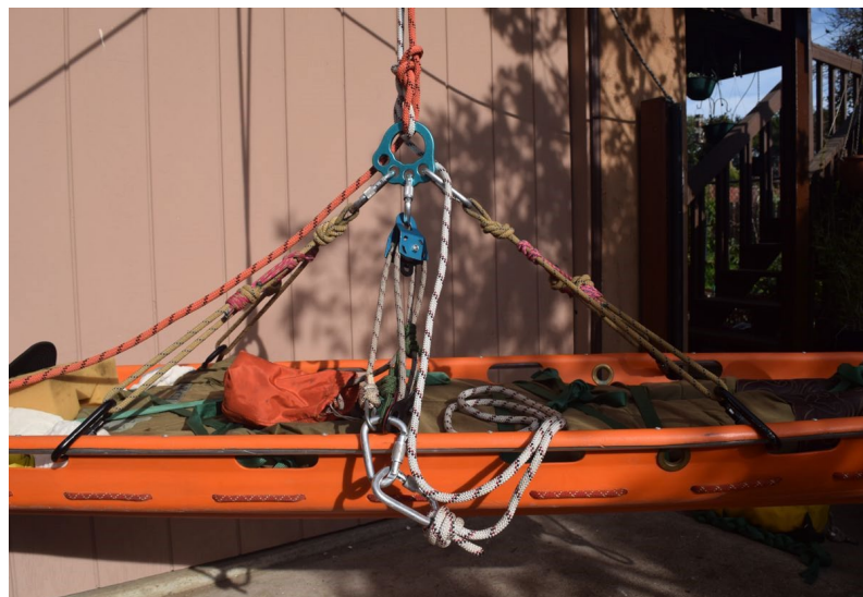
Interlocking yoke knot on rigging plate with spider and jigger attached
