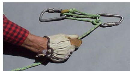
releasing a Radium 3:1 hitch
