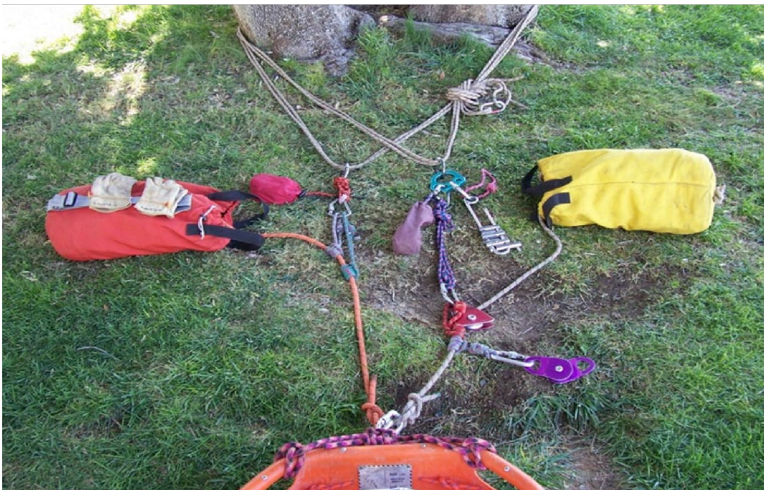
alternative anchor with traditional tensioned working rope and un-tensioned belay rope
