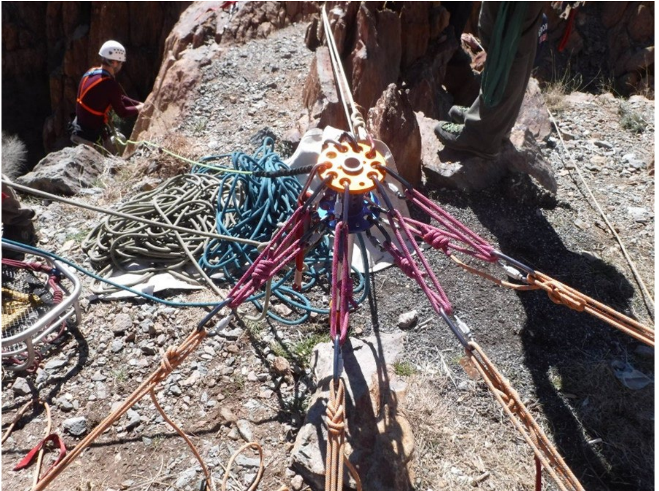
AZORB as an elevated forward focused floating anchor
