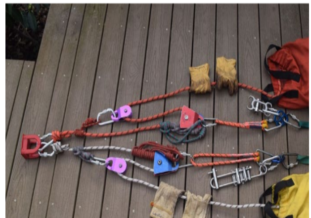
two tensioned rope system raising
